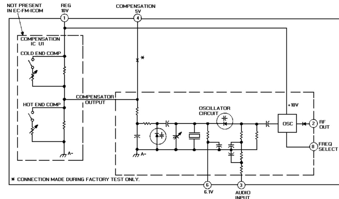
Figure 3 - Equivalent FM ICOM Circuit
