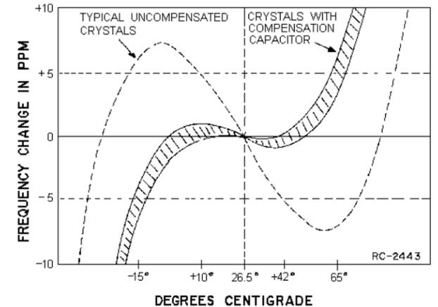
Figure 2 - Typical Crystal Characteristics
