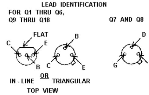
NOTE: LEAD ARRANGEMENT, AND NOT CASE SHAPE, IS DETERMINING FACTOR FOR LEAD IDENTIFICATION.
