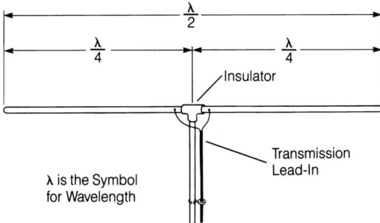
You would change a dipole antenna to make it resonant on a higher frequency by **making it shorter.**
