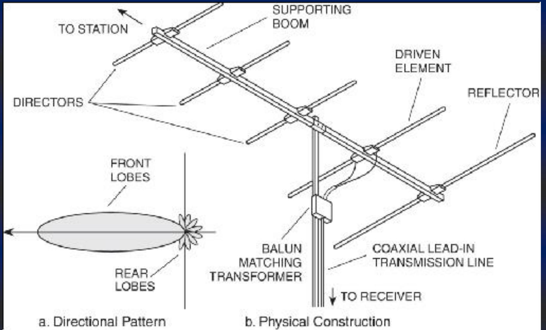
The three types of **directional antenna** that you need to know for the exam are the quad, Yagi, and dish. The one pictured above is a yagi.
