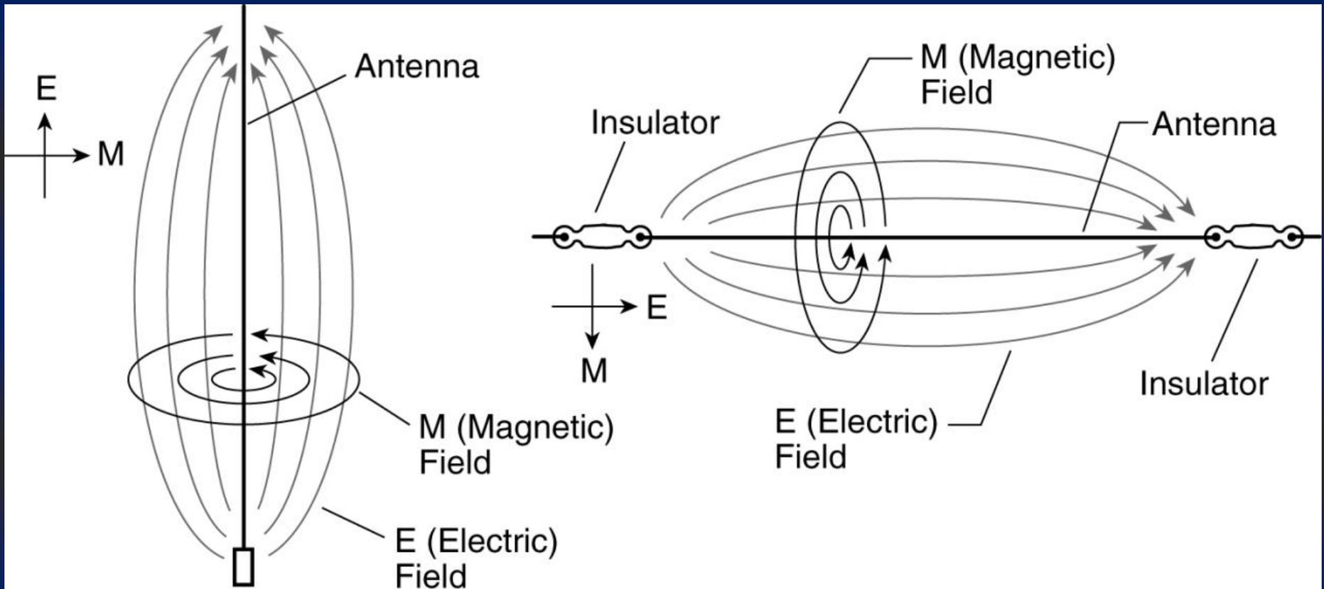
a. Vertically-Polarized Antenna
